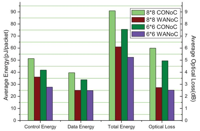
Fig. 4. Power consumption of WANoC and CONoC using 1024-bit packets under uniform traffic pattern.
