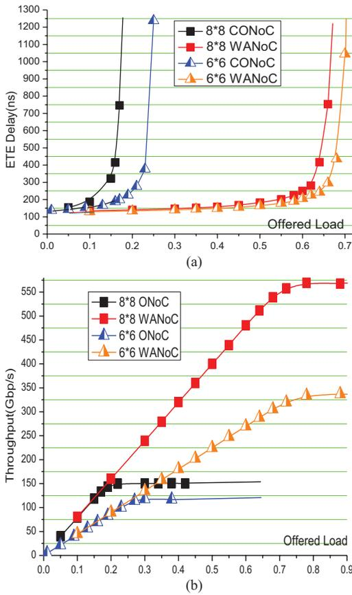
Fig. 3. Network performance of WANoC and CONoC using 1024-bit packets.
