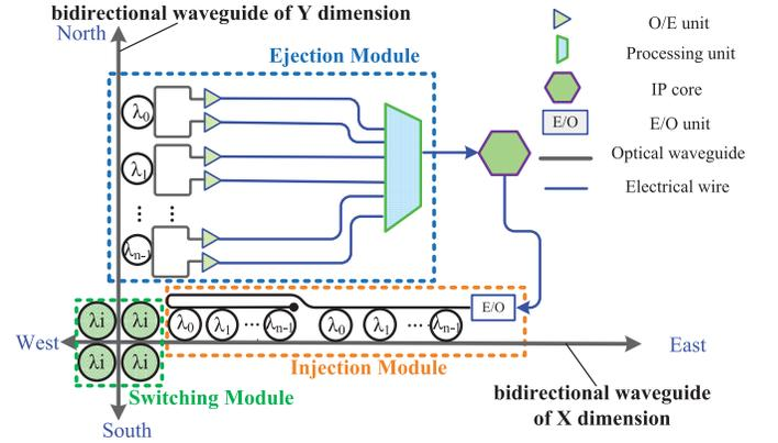
Fig. 2.  $4 \times 4$  router. IP core is connected with optical router via E/O and O/E units. Processing unit deals with multiple electrical signals, arranges the right order for them, and makes them acceptable for the IP core.
