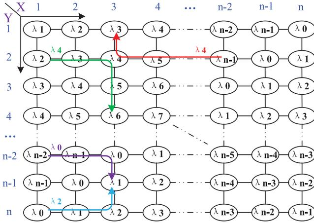
Fig. 1.  $n \times n$  WANoC. The numerical value in each node presents the wavelength assignment result.
